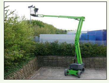
The HR17 Hybrid 4x4 also incorporates ToughCage and SiOPS technologies. A tough impact resistant composite base and larger cross-section steel give the ToughCage strength and durability, while SiOPS offers additional operator protection.
